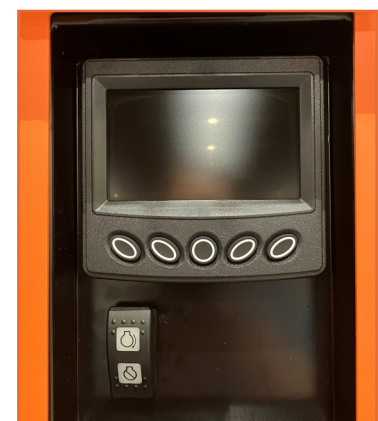
FIGURE 4-2. IGNITION SWITCH ON INSTRUMENT PANEL
